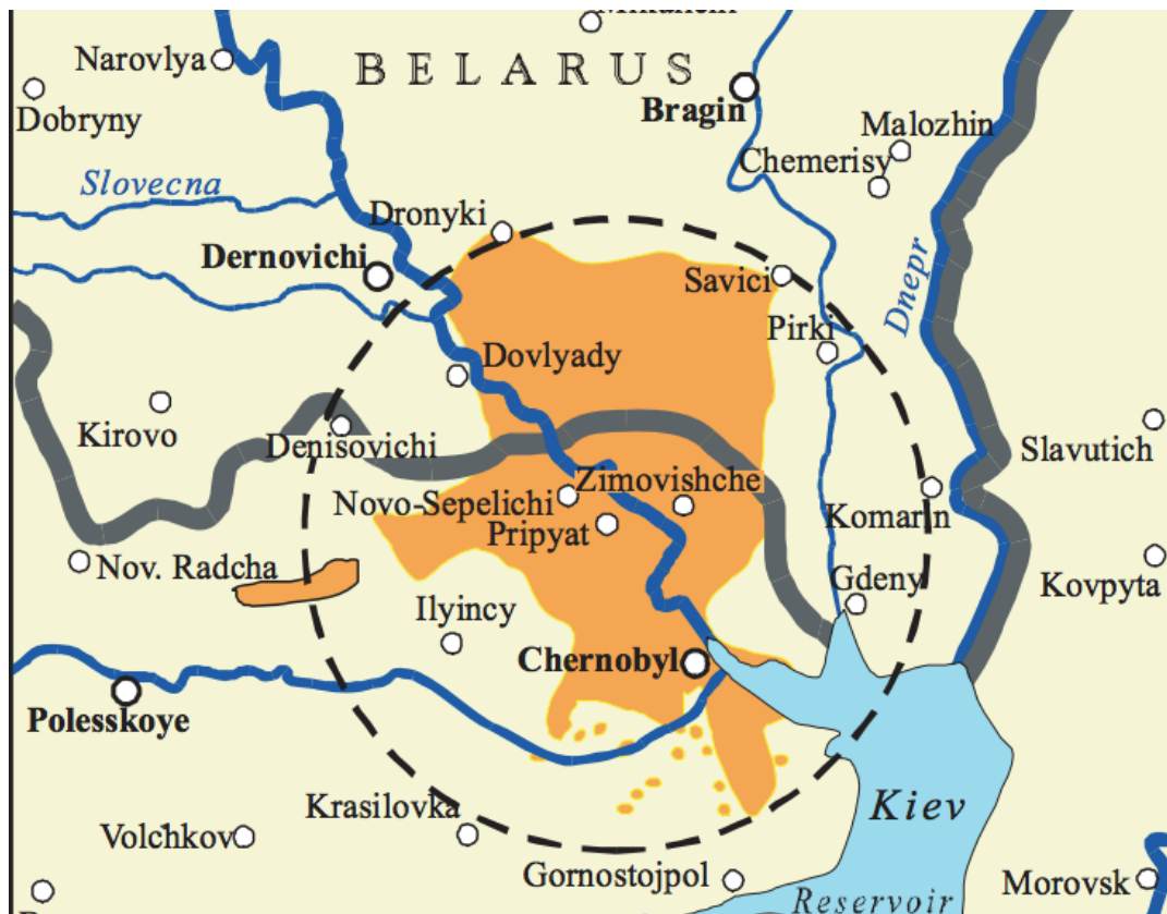
Figure 4: Map surface ground deposition of plutonium along the Pripjat river near the Chernobyl nuclear power plant: areas (orange) where the surface ground deposition of plutonium-239,240 exceeds 3.7 kBq/m 2 . Extracted from [IAEA2006b].
